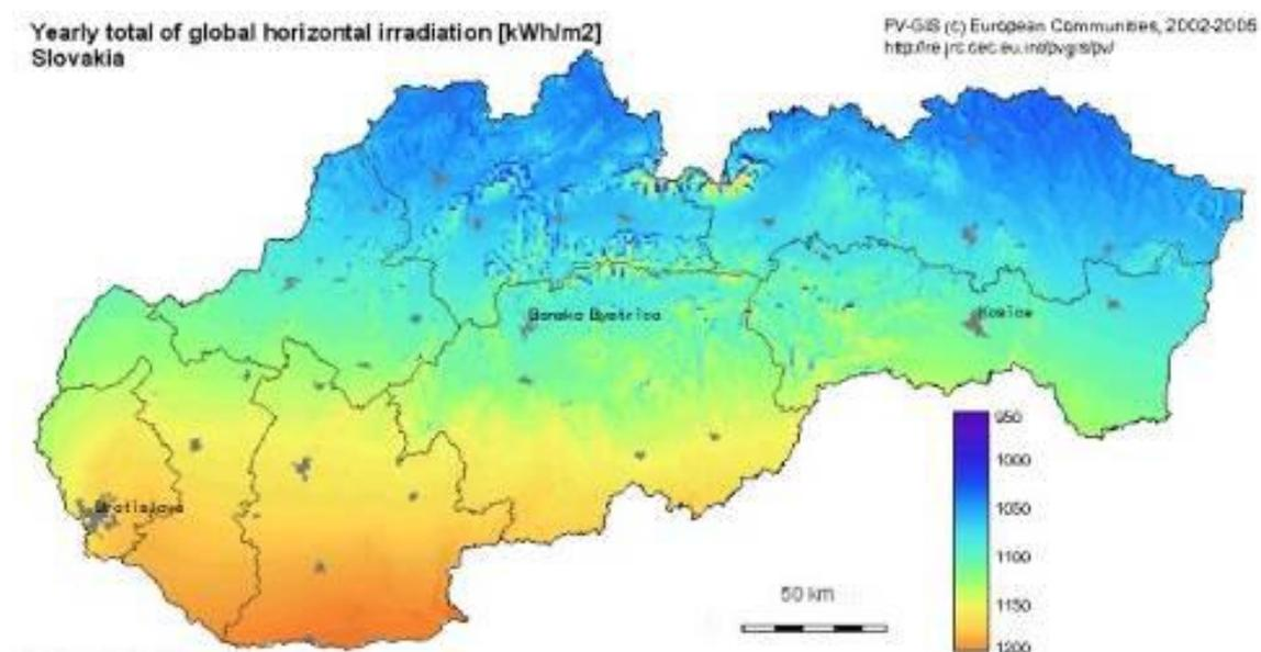
Fig. 4 Yearly global irradiance energy (incident on horizontal plane [kWh/m<sup>2</sup>])
